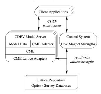
Figure 1: The RHIC/AGS online model architecture. Each running model server is a separate unix process, binding the server interface to an instance of a CME.
