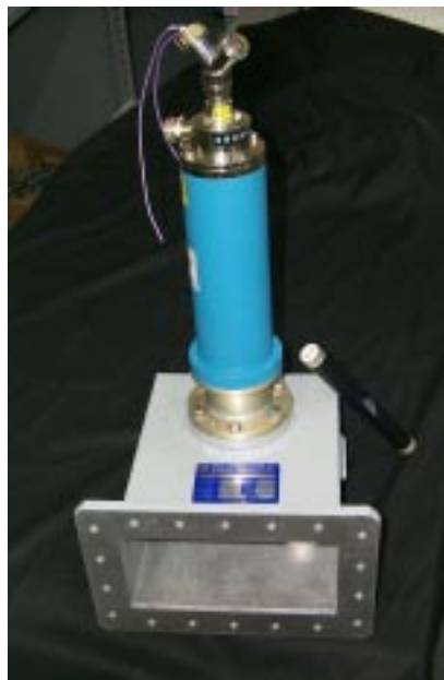
Figure 1: Photograph of the type 9725 resistive-load assembly for 850-MHz.
