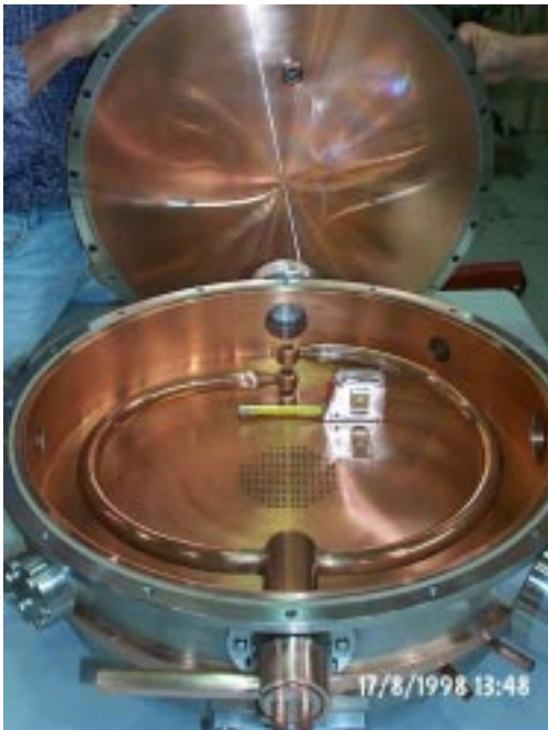
Figure 4. First DTL Buncher developed and manufactured at INR, Russia.
