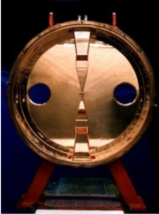
Figure 3. First DTL tank with ridges and stems installed and aligned.
