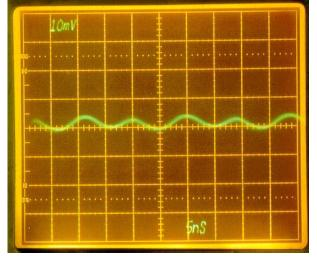
Figure 4: The measured micro-bunch current of the two RFQs demonstrate the 180° phase shift between the beam bunches. The scale is 5 ns/div. horizontally.
