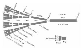
Figure 1: Layout of the 12.5...200MHz linac system for 400 mA of Bi<sup>+</sup>.
