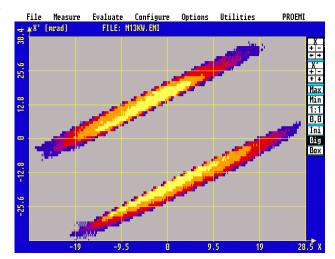
Figure 6: Measured emittances 1m behind the RFQ at the place of beam crossing. The ellipses correspond to the 90% normalized RMS-emittances which are  $\epsilon_{RMS}$ =0.107 and 0.114 mm mrad for each beam.
