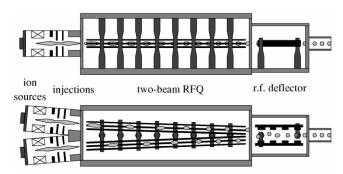
Figure 2: Experimental set-up of the two-beam funneling experiment.
