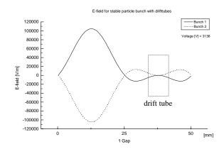
Figure 9: E-field in the funneling-deflector over the length of two cells.
