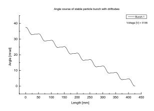
Figure 7: Motion of the stable-particle during bending in the funnelingdeflector.
