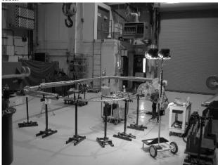
Pressurized helium flow is established through the pumped loop. Pressure, temperature, and flow rate of helium can be controlled. The loop is appropriately instrumented with temperature sensors and voltage taps. Current is measured by an external Hall probe array.
