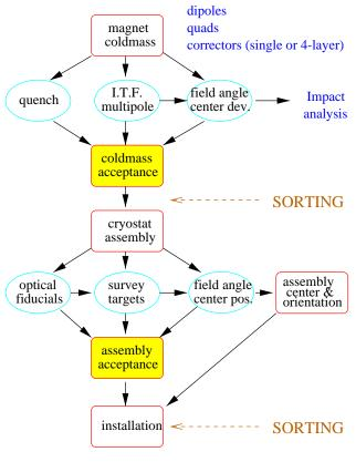
Figure 1: Magnet acceptance and sorting procedure.
