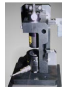
Fig. 8 Laser finder on calibration fixture
