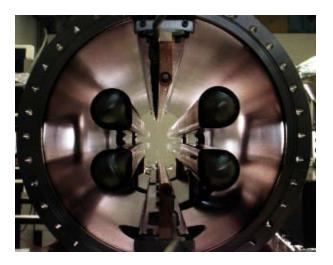
Figure 2: The electrode structure of the CESR separators.
