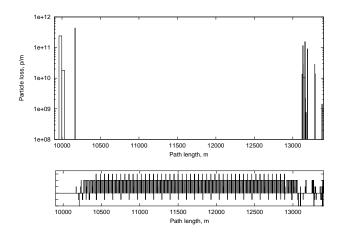
Figure 3: Beam loss at unsynchronized abort at collisions.
