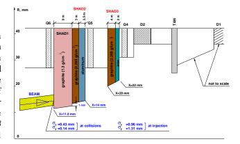
Figure 4: Shadow collimators in the IP5 outer triplet.
