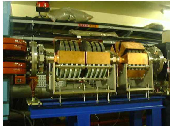
Fig.1 Impedance tuner installed in the KEK PS.
