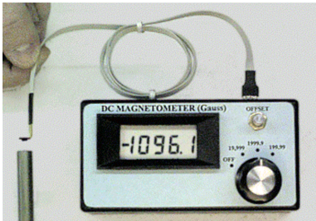
Figure 2. Photo of the DC gaussmeter.
