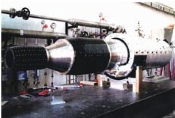
Figure 7: One of the KLOE low- \beta triplets on the alignment bench.
