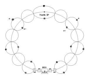
Figure 4: Pretzel Scheme with 7 bunches on BEPC
