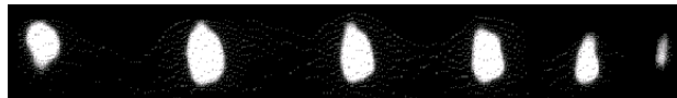
Figure 7: The synchrotron light of the accelerated beam within the turns 4 to 10 (from right to left)
