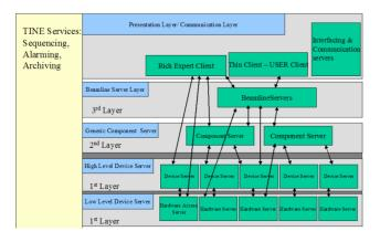
Figure 2: Beam line control layer concept
