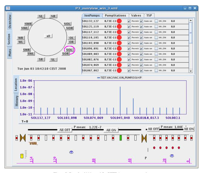
Figure 3: Running jddd panel for PETRA vacuum controls.
