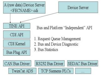
Figure 1: Architecture of the Common Device Interface
