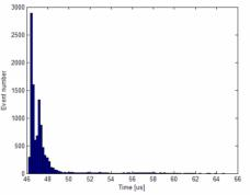
Figure 3: The latency time of a FESA RT action is well distributed below  $50\mu s$  on a VME RIO3 800 MHz controller.
