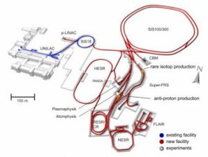
Figure 1: Layout of the FAIR facility including the existing accelerators UNILAC and SIS18.
