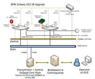
Figure 4: Scheme of the planned SIS18 BPM system to test and demonstrate the usability of FESA.
