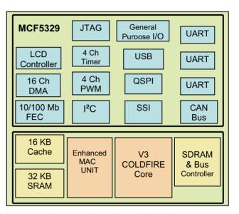
Figure 1: The MCF5329 block diagram.
