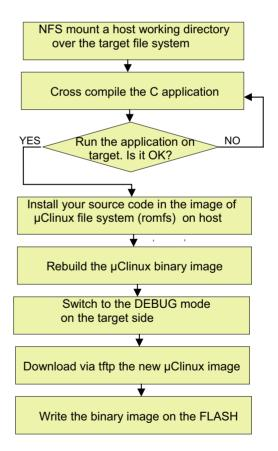
Figure 3: The software development flow.
