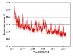
Figure 5: Measurement result of E-069 without connecting the shields of the lead lines to the E-069 analog ground.
