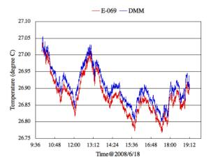
Figure 3: Measurement results of E-069 in comparison with DMM.
