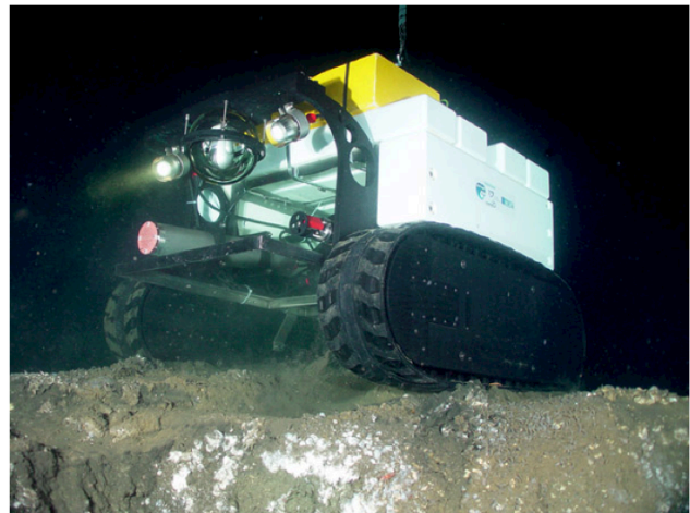
Figure 2: A small tethered vehicle on track. It can roam within 50 m from its central position. It is equipped with various physical and chemical sensors and a camera.
