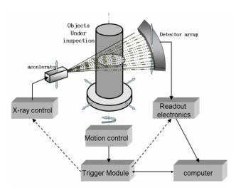
Figure 1: typical schematic block diagram of industrial CT.
