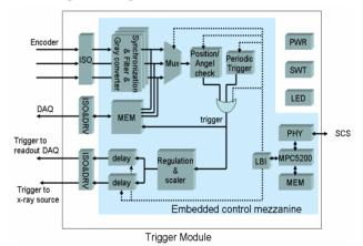
Figure 2: Functional block of trigger module.
