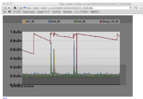
(b) A typical example of data browsing stored in the SQL server. In the present data browsing system, the graphs are generated by “PHP/SWF Charts” available from maani.us[6].
