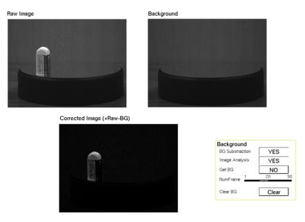
Figure 3: Subtraction of background from raw image. The left side of the upper image shows the raw data. The right side of the upper image shows background data. The result of subtraction is shown in the lower image.
