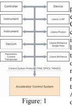
There are auite parameters that define environment in which the Control System operates. We can find heterogeneous with instruments different levels of complexity. Beside that the equipment is distributed over large remote regions and needs to provide reliable access regardless of the distance from the control room (see Fig. 1). Another characteristic of such operating environment is that the control is centralized, but
