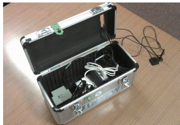
Figure 5: The in-vehicle unit of KURAMA-II. A CsI detector and a CompactRIO are compactly placed in a toolbox with the size of 34.5 cm 17.5 cm 19.5 cm.
