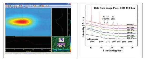
Figure 3: X-ray beam 2-D map and data for sample LaB6 at different pressure.
