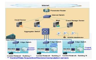
Figure 1: Distributed Architecture Control Network.
