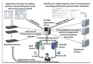
Figure 4: Conceptual block diagram of the DCOMS.
