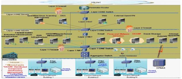
Figure 2: Securely designed modern day Distributed Architecture Control Network.
