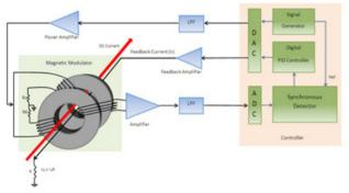
Figure 6: Magnetic modulator in a closed loop – low frequency channel of DCCT.
