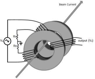
Figure 1: Schematic of second harmonic magnetic modulator.
