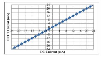
Figure 8: DCCT output vs. input DC Current.
