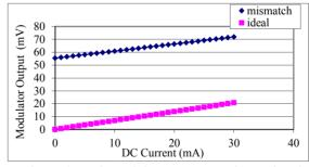
Figure 4: Peak modulator output vs. input signal.
