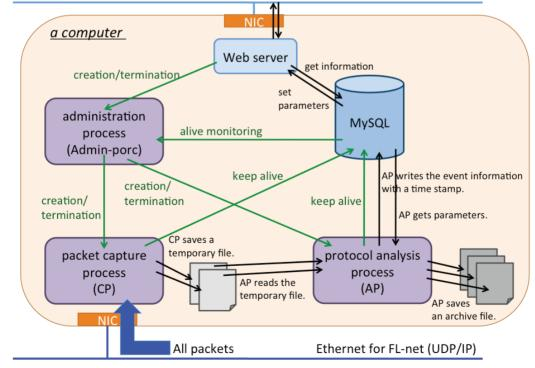
Figure 3: Schematic view of the monitoring system for the FL-net protocol.
