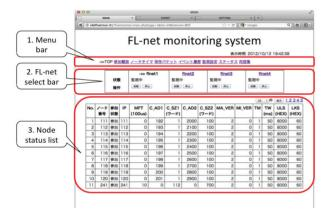
Figure 4: The main page of the Web browser. The language is set to Japanese. The red line around the box No. 1 area indicates the menu bar used for browsing The No. 2 area is the FL-net select bar, which can start/stop the monitoring by the click of a button Finally, the No. 3 area shows the node status and configuration list.
