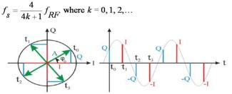
Figure 2: I/Q detection scheme.
