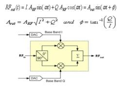
Figure 6: Typical Block diagram of I/Q modulator.
