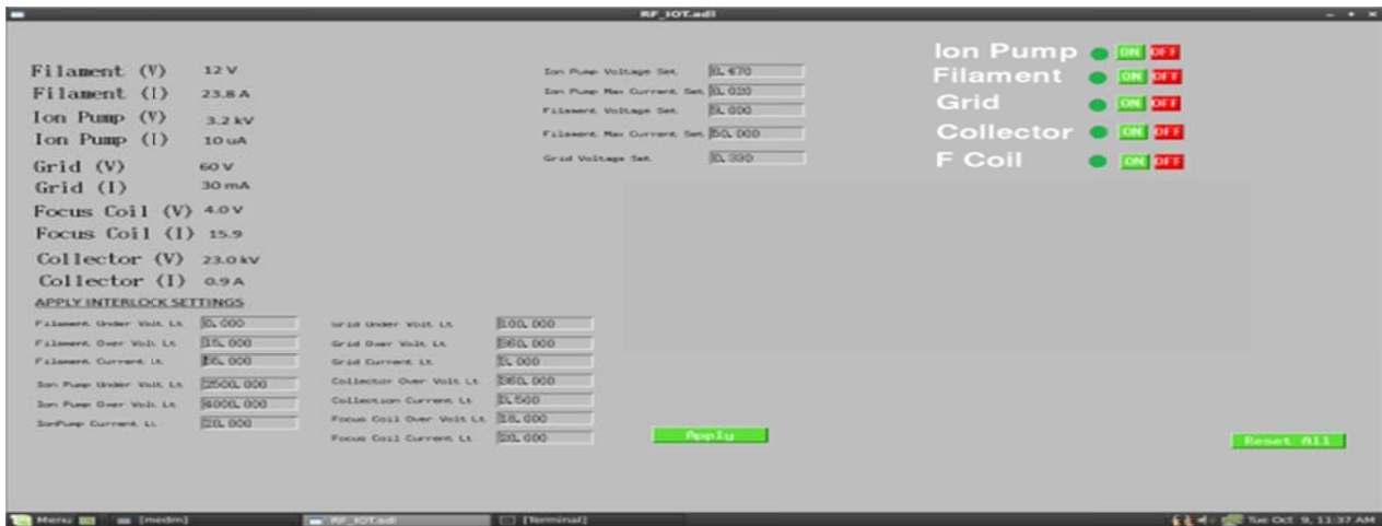
Figure 4: GUI for Remote operation.
