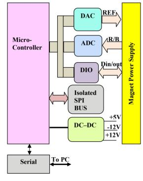
Figure 2: Block Diagram of Slave Controller.
