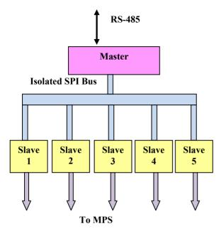
Figure 1: Block Diagram of proposed Magnet Power Supply Controller (MPSC).
