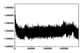
Figure 3: Voltage Drift vs. Time for enclosed systems.
