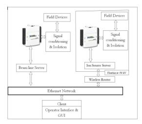
Figure 2: Control System Architecture.
