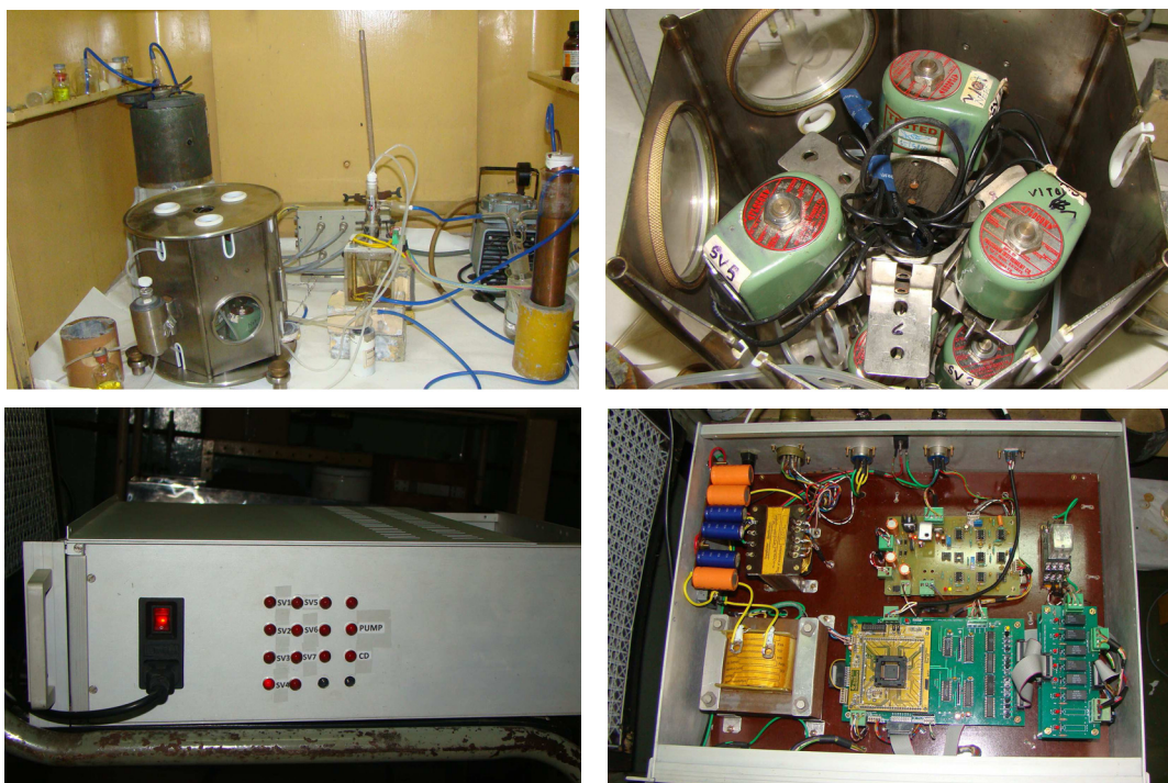
Figure 2: Hardware assembly consisting of (clockwise from top left) Process Assembly in fumoid, Solenoid Valve Assembly, Electronics Assembly inside the 19" Controller rack, Front panel of Controller Unit.
