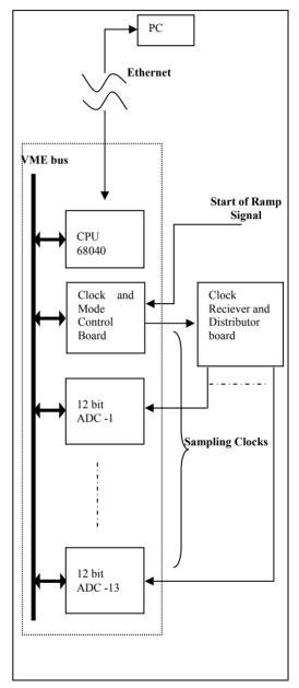
Figure 1: Scheme of Data Acquisition System.
