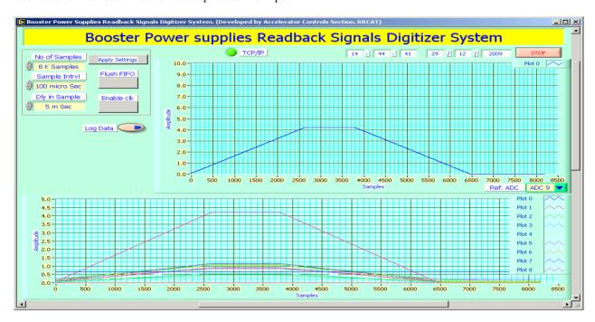
Figure 2: Graphical representation of captured ramp data waveforms.
