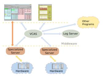
Figure 2: Control system schema.
