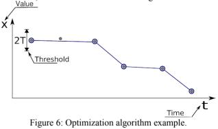
This algorithm allows to reduce the rate of data growth from 3.4 MB/day to 1.28 MB/day per channel.
