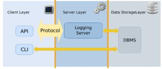
Figure 3: Logging system architecture.
