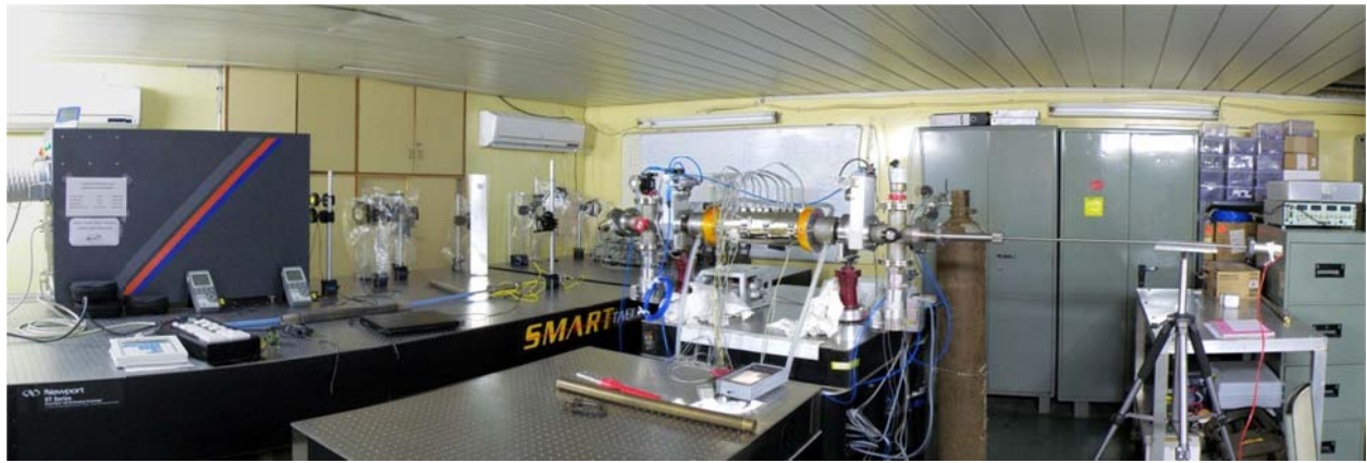
Figure 12: View of the plasma accelerator laboratory showing the ArF laser and the plasma accelerator chamber.
