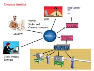
Figure 2: Common interface for handling beamline components using STARS.
