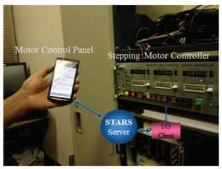
Figure 6: Stepping motor controller operated by the Motor Control Panel through STARS.
