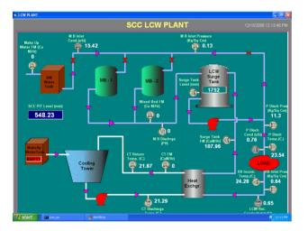
Figure 3: GUI for SCC LCW plat monitoring system.
