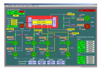
Figure 2: GUI for SCC Vacuum control system.
