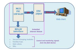
Figure 1: Block schematic of the control architecture.
