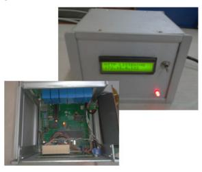
Figure 5: Complete assembled module.
