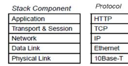
Figure 2: TCP/IP stack and the protocols used
