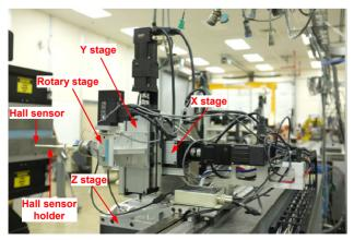
Figure 1: Hall probe measurement system.
