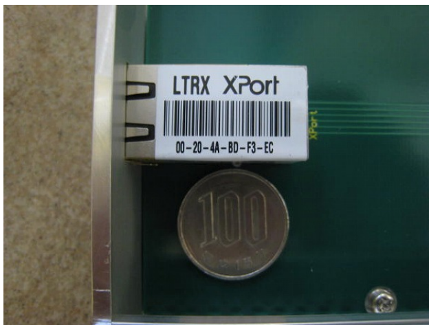
Figure 1: XPort module mounted on a board.
