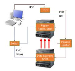
Figure 4: Shelf level test demonstration setup.
