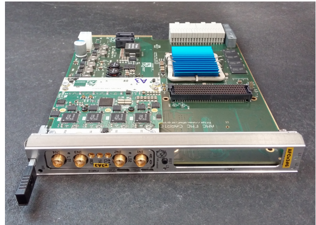
Figure 2: AFC v3.1 with FMC130 mounted.
