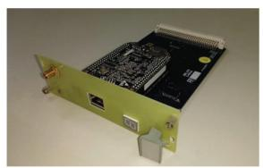
Figure 1: The new local controller prototype.
