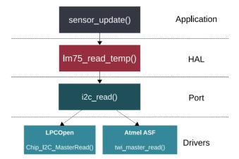
Figure 2: openMMC sensor update function call sequence.
