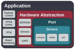
Figure 1: openMMC firmware structure.
