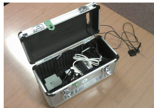
Figure 2: In-vehicle unit of KURAMA-II. A CsI detector and a CompactRIO controller are compactly placed in a tool box with the size of 34.5 cm × 17.5 cm × 19.5 cm.
