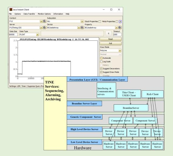
The Client software is LabVIEW based and connects through TINE to the device servers.
