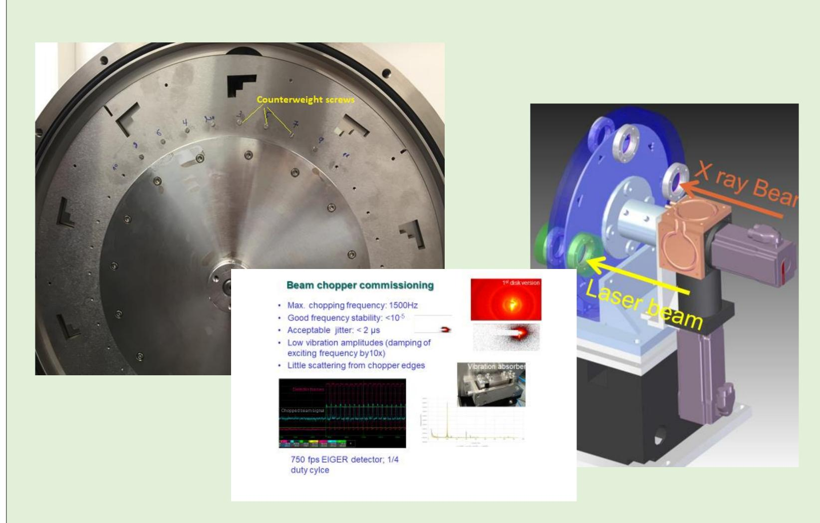
Velocity stabilization of the chopper is archived by the velocity control motion mode of the TwinCAT NC. The motor follows the output frequency of the AX5106 Motor controller which is integrated inside the TwinCAT NC. The motion stability is observed by the diagnostic laser diode and the motor controller output frequency is corrected inside a feedback loop based on the diagnostic signal.
