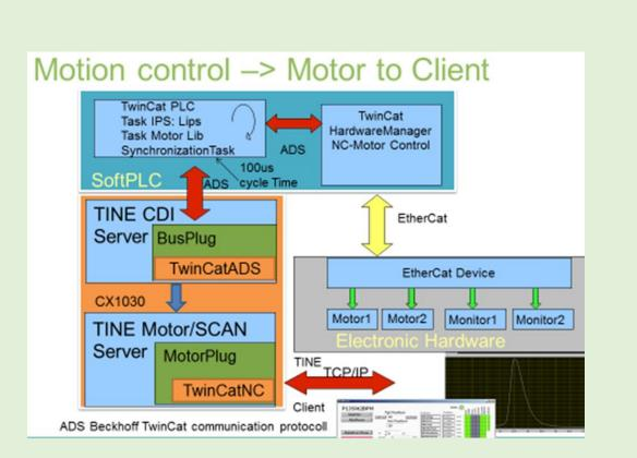
The Client software is LabVIEW based and connects through TINE to the device servers. The Client allows motion control of the Chopper for rotation speed, wheel positioning in angle and position. The Timing GUI is used to set device triggers and delays of connected beamline devices like the detector, laser, sample changer, shutters,...
