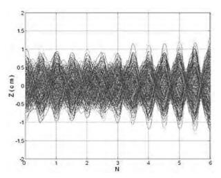
Figure 7: Axial trajectories of  $H^-$  ions (I = 0 mA).
