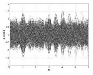
Figure 8: Axial trajectories of  $H^-$  ions (I = 30 mA).
