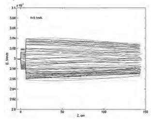
Figure 2: Beam energy vs distance from buncher (taking into account space charge effects).
